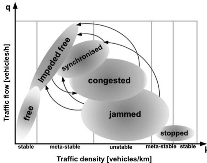
Figure 1: Transition from traffic situations with flowing traffic ('impeded' free flow and synchronized traffic) and congested traffic (according to Kim (2002), Page 21)
