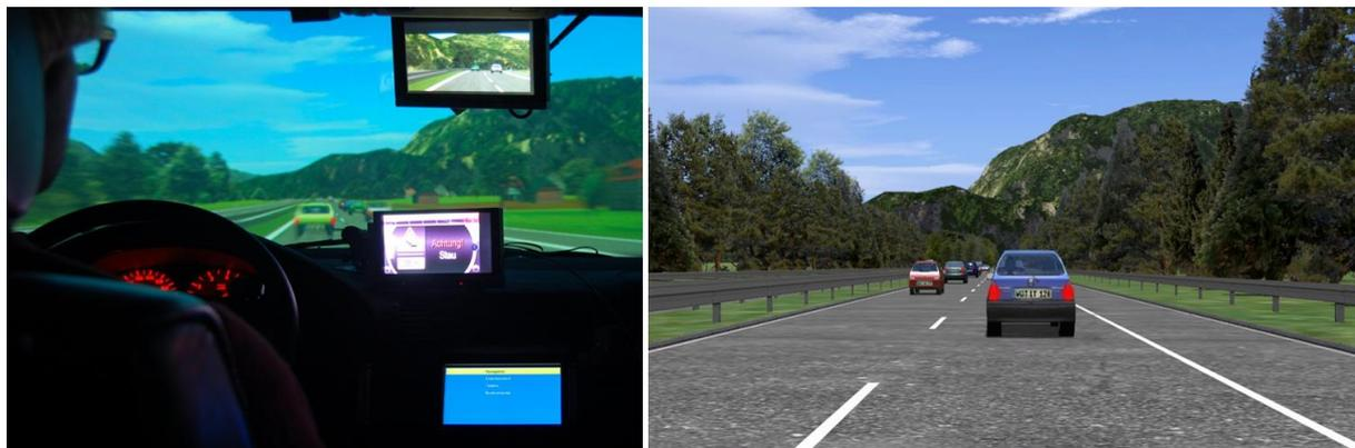
Figure 3: Driver's cabin of the driving simulator with view of the screen in the center console (left). Screenshot of a driving situation while approaching the tail end of a congestion (right)
