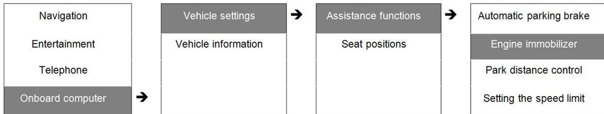
Figure 4: Flowchart of the navigation in the menu system for the task 'Activating engine immobilizer'
