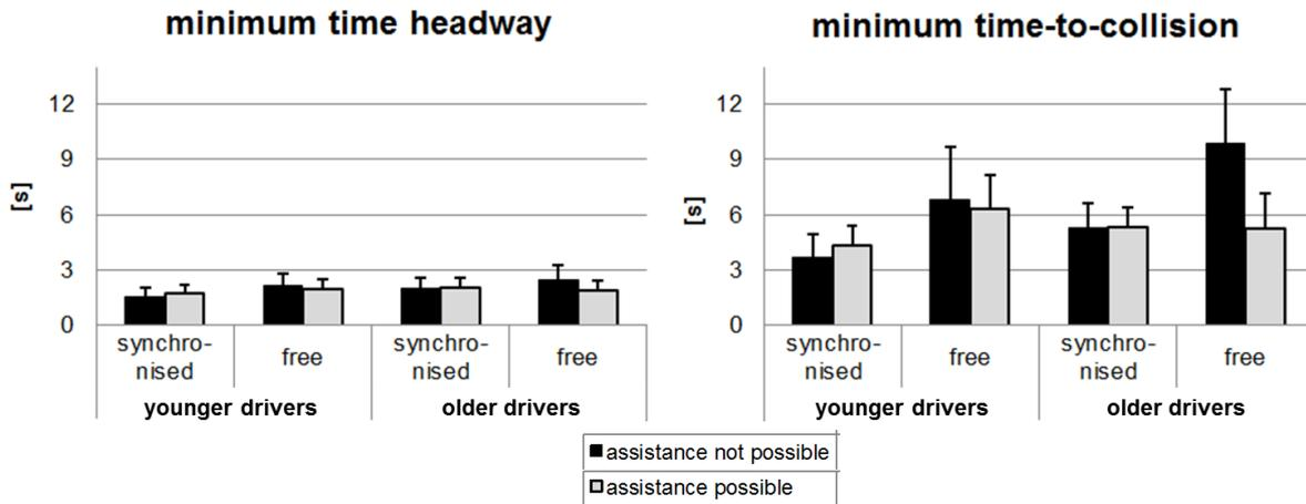
Figure 7: Minimum time headway (left) and minimum time-to-collision when following another vehicle (right). Here, mean values and standard deviations are illustrated
